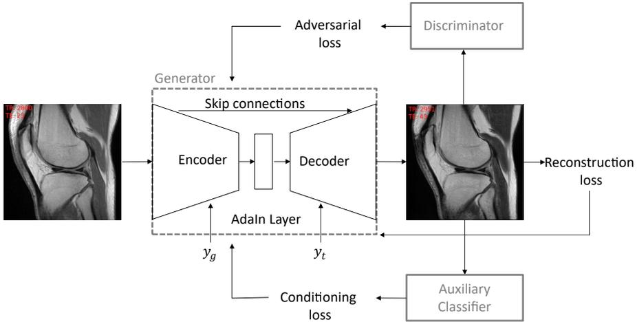
**Fig. 1.** Training procedure of our approach: The generator receives a real input image (left image), including its acquisition parameters TR and TE ( $y_g$ ) as well as the target acquisition parameters ( $y_t$ ) and translates the image to the synthesized target contrast (right image). The discriminator learns to distinguish between real and synthetic MR images, and the auxiliary classifier is pre-trained to determine the acquisition parameters from the image.
